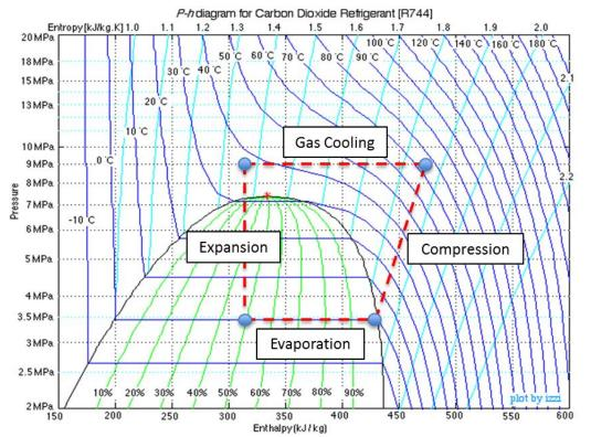
Transcritical cycles absorb heat within the vapor dome (subcritical) but reject the heat above it (supercritical). For a supercritical fluid, temperature is decoupled from pressure. Cooling capacity performance  $(\Delta H_{EVAP})$  improves as  $T_{GC,exit}$  approaches the ambient. As a result, the gas cooler should be as effective as possible without creating excessive pressure drop (an optimization opportunity).
