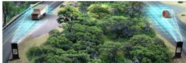
The Poles setup at two ends of the hair pin bend detecting incoming traffic
