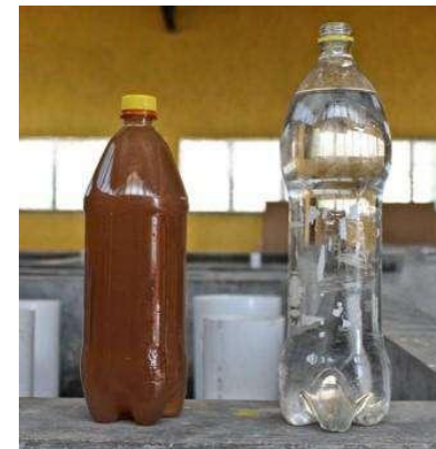
Water entering an AguaClara plant (left) for treatment, compared to water leaving an AguaClara plant (right) after treatment.
