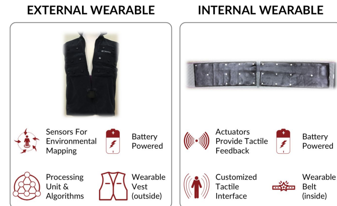
Figure: The two components of the Eyeronman wearable. Source: Tactile Navigation Tools
