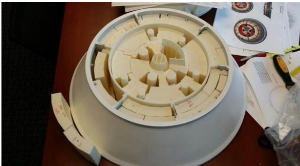
(a) The buoy contains hundreds of solid foam blocks that keep it afloat in water. The Stones team used a 3D printer connected to their computer design system to produce scaled-down plastic versions of all components in only four weeks.
