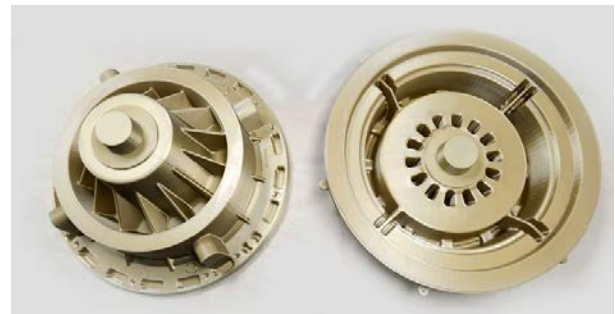
3D-printed gearbox prototype and sand molds by Oak Ridge National Lab. Source: NREL .
