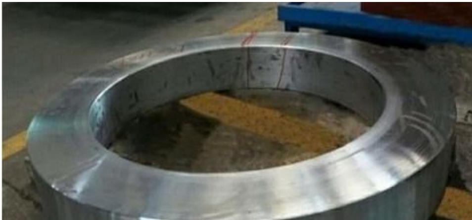
3D-printed pressure vessel cylinder by Nanfang. Source: 3Ders .
