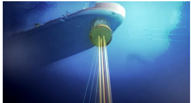
b) The connecting system features a huge buoy 19 metres tall, moored at the surface, which receives oil and gas from the seabed. The buoy slots into a turret inside the FPSO, like a plug and socket, enabling production while holding the vessel safely in place. By 3D printing the system in miniature, the team could show how it allows the FPSO to turn and remain stable in rough seas and disconnect when the wind and waves become too strong, helping the vessel and crew stay safe. Source: Shell .
