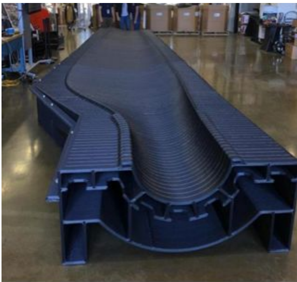
Image of a 3D-printed turbine mold at Oak Ridge National Laboratory. Source: Make Parts Fast
