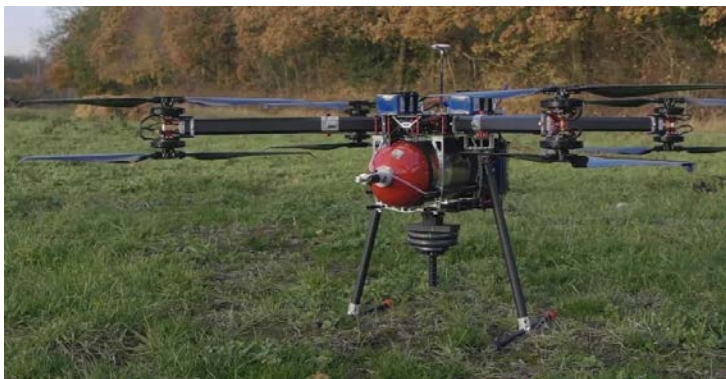
Model drone equipped with a 6-L Hydrogen Cylinder. Source: Drone Life
