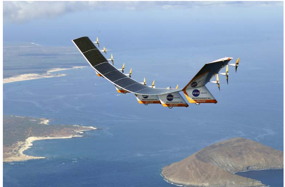
NASA's solar-electric Helios prototype using solar PV technology in the daytime and RFC technology at night.
