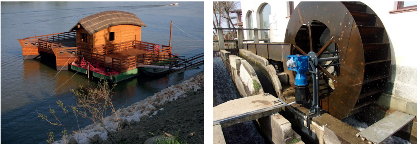
■ ■ ■ FIGURE 6 Floating water wheel (AIAMS, Silvano Bonaiuti) on the left, and gravity water wheel (breastshot type) on the right (Marco Gatta).
