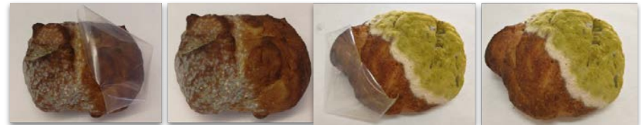
Figure: NanoPack active packaging extends bread shelf life by 3 weeks. A first round of antimicrobial efficacy tests proved NanoPack film's ability to inhibit mold growth on food-additive free bread. The bread that was inoculated with mold spores and packed with NanoPack innovative film insert had no mold growing in the area exposed to the film for up to 27 days post packaging.
