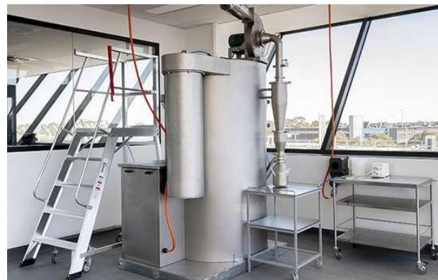
Figure: A pilot scale spray dryer in the Monash University food grade lab. Credit: Monash
