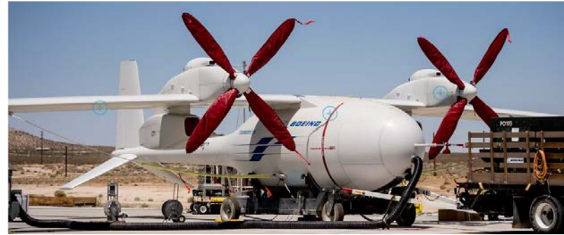
Phantom Eye achieves an altitude of 65,000 ft, with endurance of 4 days at 65,000 ft (19,800 m). Source: Boeing.
