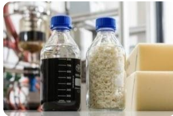
Figure. BASF's process breaks down the flexible polyurethane and delivers the initially used polyol. Source: BASF.
