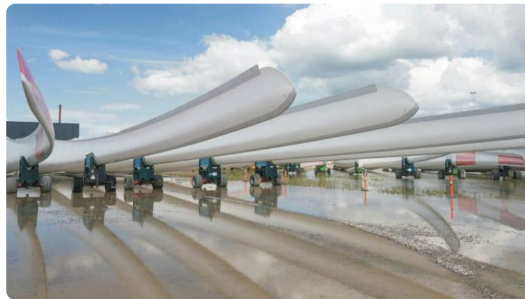
Figure. The first six 81-meter long recyclable blades. Source: FT.
