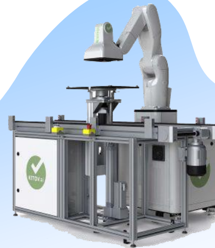
CorePlus showing the robotic are and rotating table. Arm robot equipped with camera can scan all the angles and heights. Source: kitov.ai .
