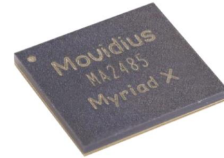
Figure 1. Movidius Myriad X VPU: Real-time DNN inferencing with 1 TOPS performance and 700Mpps image signal processing. Source: Myriad .
