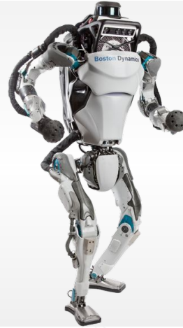
Atlas by Boston Dynamics: Whole-body mobility and bimanual manipulation
